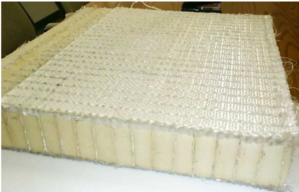
Figure 2. Portion of 3"-thick hybrid TYCOR FRF core.
